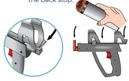
Press the arrow to move the guide forwards and position the spray nozzle correctly in contact with the orange spray piece.
