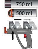
Put the bottom of aerosol between the rib and the back stop.
